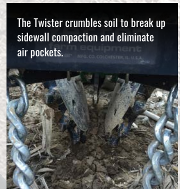
With help from the 6200 Drag Chain, the Twister Poly Closing Wheel creates a consistently closed seed trench.
