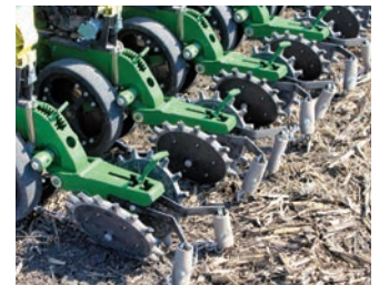
A Twister Closing Wheel can be installed in as little as five minutes.
