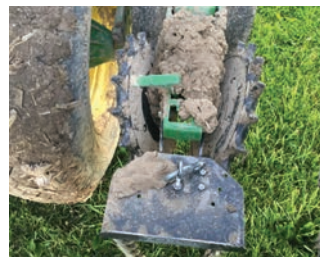
The Twister's rounded center design prevents mud buildup.
